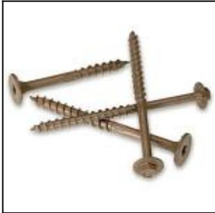
The Strong-Drive SDWS Timber screw is designed to provide an easy-to-install, high-strength alternative to through-bolting and traditional lag screws. The Strong-Drive SDWH Timber-Hex SS screw provides a structural wood-to-wood connection, including for ledgers. As all Type 316 stainless steel fasteners, the Strong-Drive SDWH Timber-Hex SS screw offers maximum corrosion protection.
